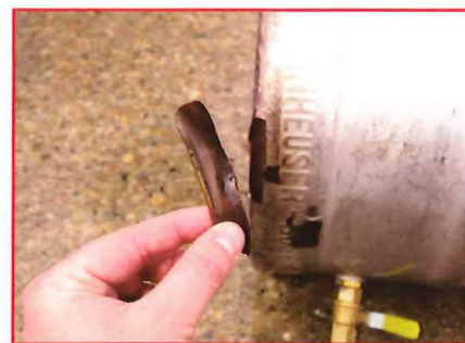
This kettle made from a used keg did not have holes in the bottom rim. The result: an explosion from pressure.
