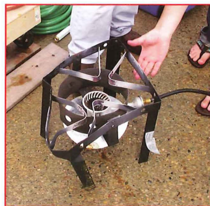
Burner damaged by exploding keg.
